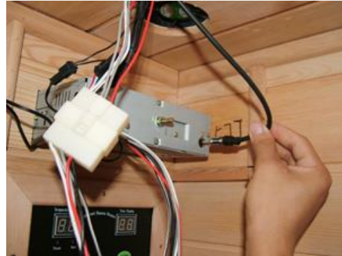
FIG-21 Link the antenna connectors
