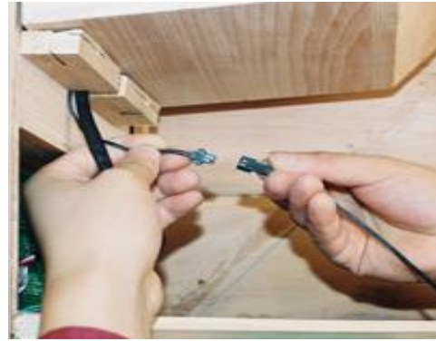
FIG-19 Link the sensor connectors
