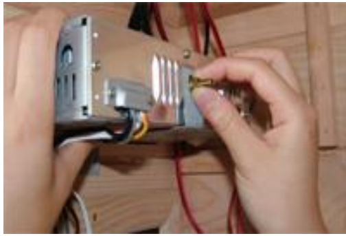
FIG-13.3 Lock the CD with its metal support
