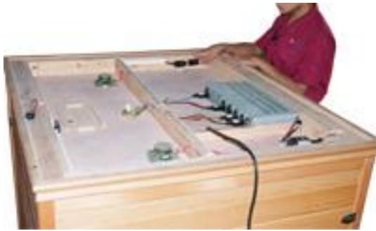
FIG-16 Connectors on the internal top board
