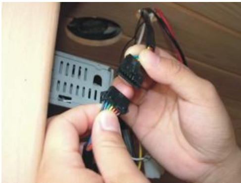
FIG-20 Link the control panel connectors
